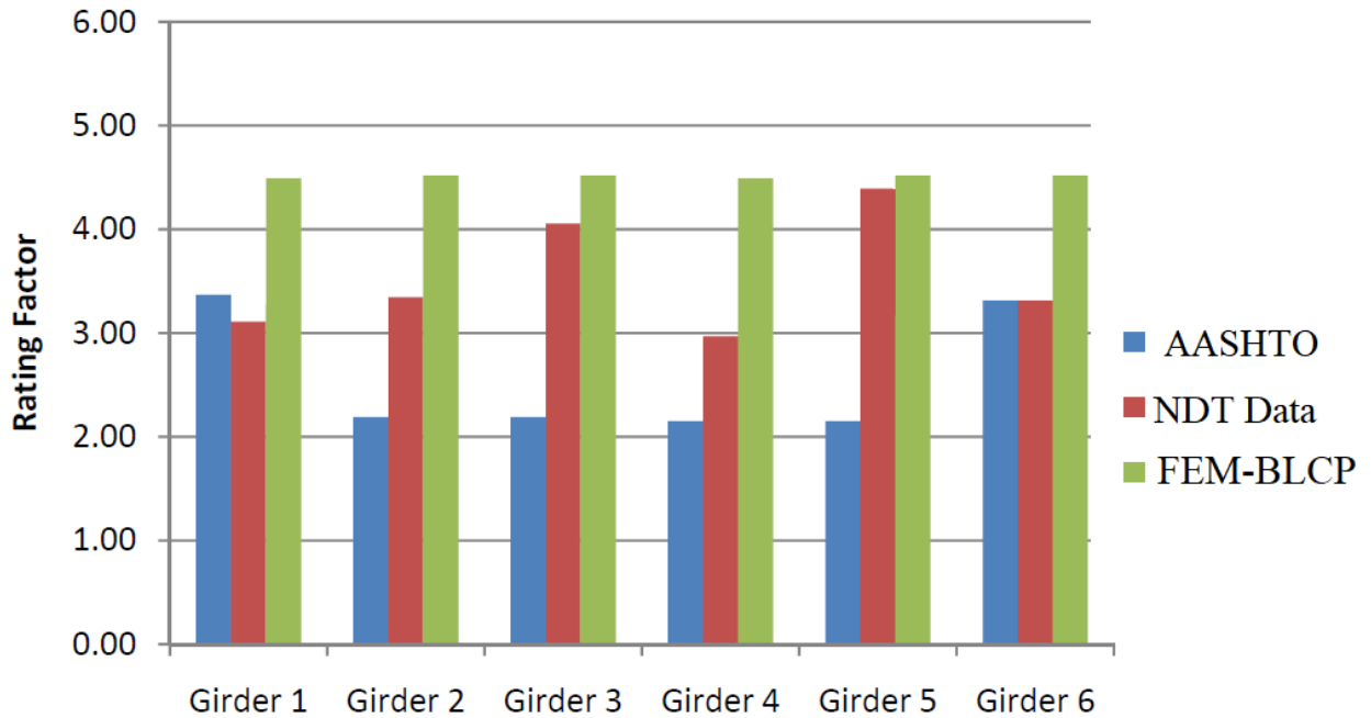
Figure 3.3 Rating factor comparison of the AASHTO approach with NDT data and the novel BLCP.
